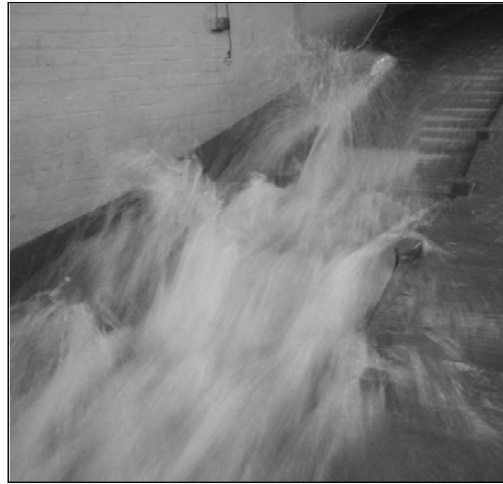
Figure 7. Model test results at PMF – effects of the architectural pillars
